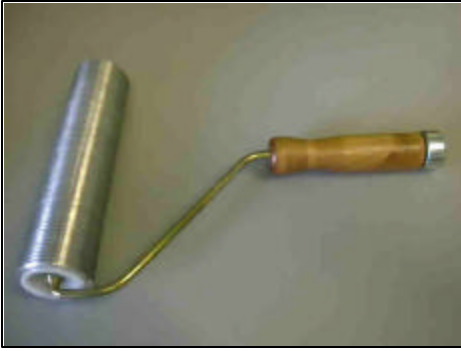
Fig. 5 – A laminating roller can make installations onto high temperature surfaces much easier. This tool can also be used on large flat surfaces where Stricture Banding™ cannot be effective.
